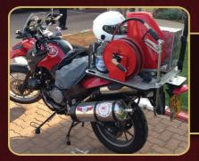
Enforcer 3 is lightweight, easy to carry, and is handheld or installs easily. Converts 3 gallons of water to 60 gallons of finished foam with a 45ft spray over 1 minute. Nitrogen or SCBA.
