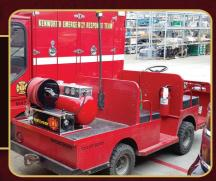
Enforcer 60 allows for 1200 gallons of finished foam from 60 gallons of water with a 95ft spray over 6 minutes. UL 711 certified.
